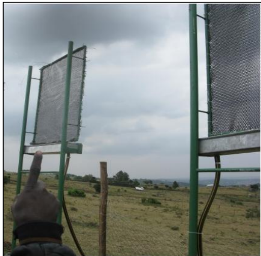
Figure 1. Fog harvesting equipment at Olteyani, Kajiado County of Kenya (ORSAM, 2013).
